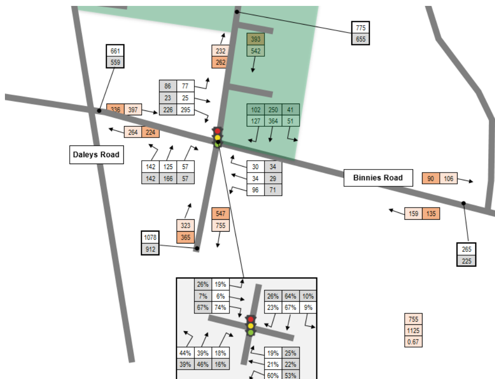
Figure 2.5 – Road 1 / Binnies Road Intersection Traffic Flows (Ultimate Scenario based on the Two-way Daily Flows Extracted from Jacobs model).
